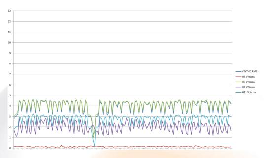
Picture 17: Harmonic distortion for Voltage % recordings in the electric network of ELPE's CC plant department after SEMAN's project
