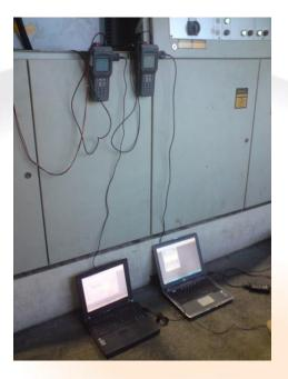
Picture 7: Measurements with special power quality analyzers and laptops
