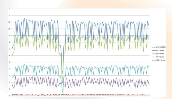
Picture 9: Harmonic distortion for Voltage % recordings in the electric network
