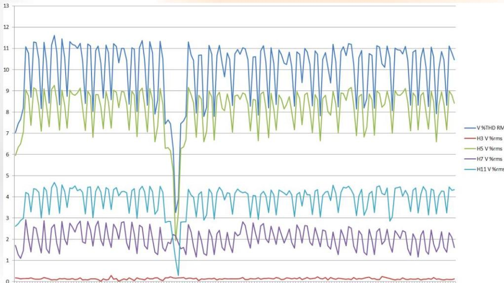
**Picture 9: Harmonic distortion for Voltage % recordings in the electric network**
