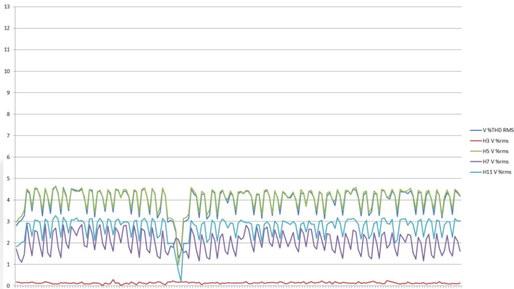
**Picture 17:** Harmonic distortion for Voltage % recordings in the electric network of ELPE's CC plant department after SEMAN's project
