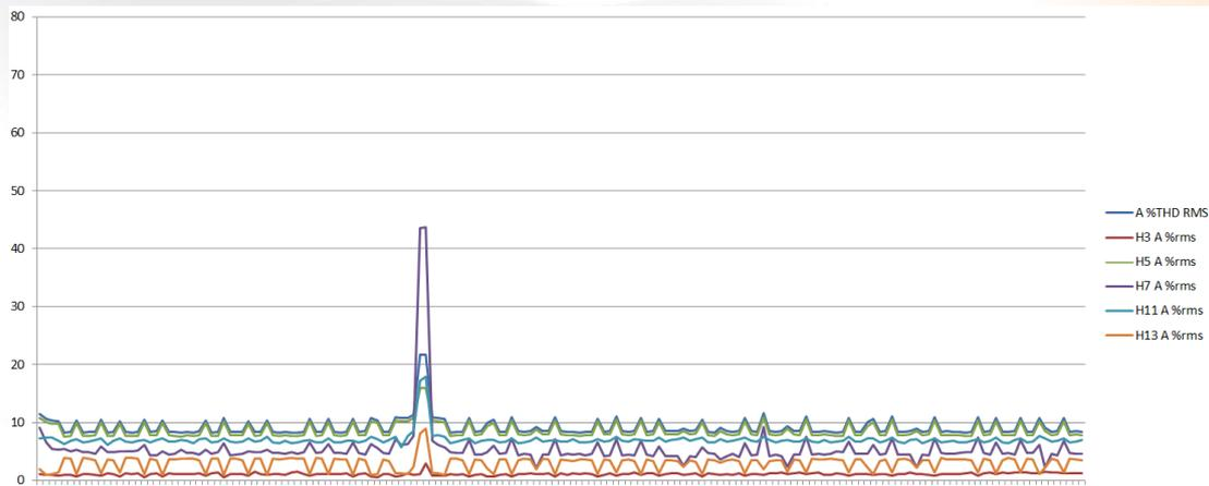
**Picture 16: Harmonic distortion for current % recordings in the electric network of ELPE’s CC plant department after SEMAN’s project**
