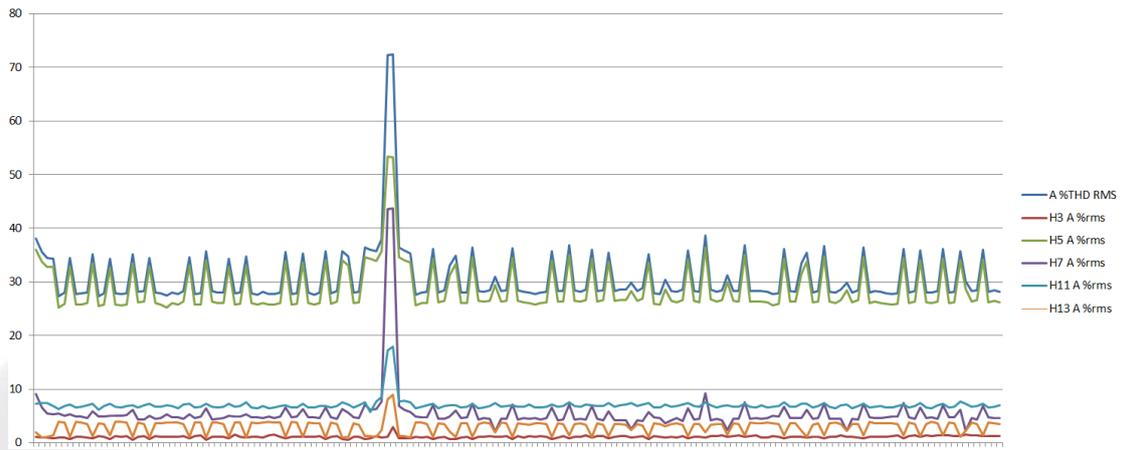
**Picture 8: Harmonic distortion for current % recordings in the electric network**
